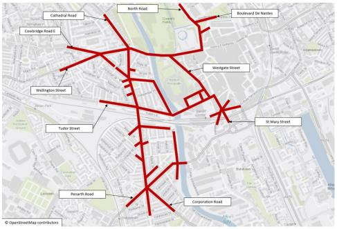
1.5 The Vissim model covers the extent shown in red in **Figure 1-1**. The results obtained from the model show the impacts of the scheme within this extent and cannot show further impacts on the wider network.
