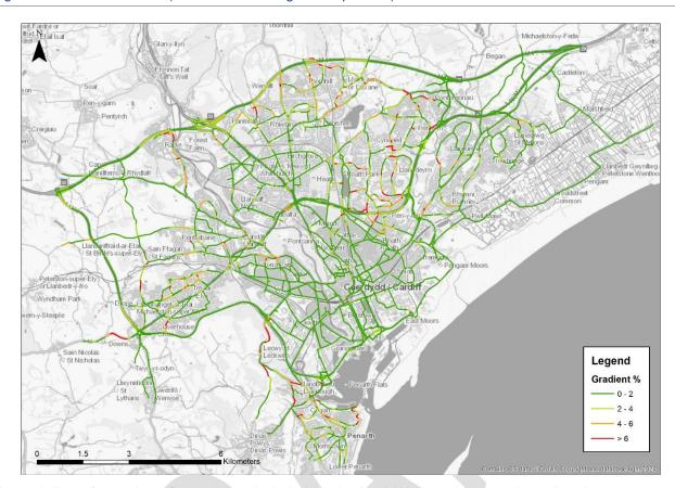
Figure 2-2 Gradient effects (absolute value of gradient percent)
