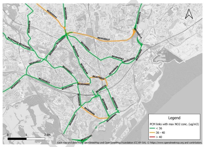
Figure 5-1 shows a mapped projection of the data shown in Table 5-1, where the entirety of the PCM road link has been assigned the maximum 2022 baseline NO<sub>2</sub> value, sampled along that section of road link.
