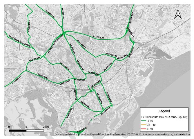
Figure 5-3 shows a mapped projection of the data shown in Table 5-1, where the entirety of the PCM road link has been assigned the maximum 2024 do minimum  $NO_2$  value, sampled along that section of road link. The figure shows that all PCM links are expected to fall below 36  $\mu$ g/m³ including along Castle Street.
